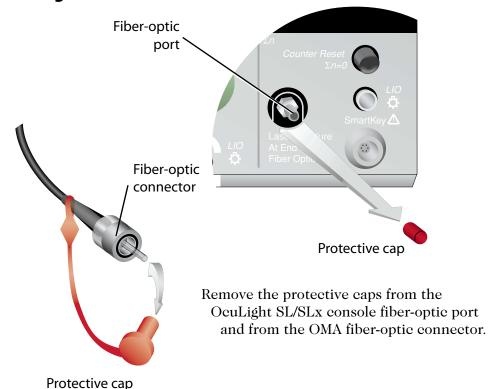
Carefully insert and finger-tighten the connector into the OcuLight SL/SLx
